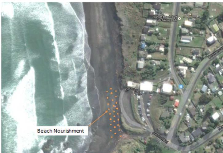
Figure 23: Diagram of Potential Beach nourishment at Port Waikato
