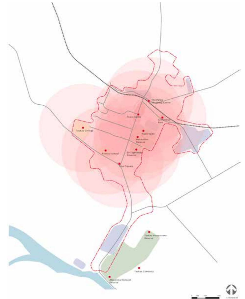
Figure 2. Walking distances from key amenities (400m walking circles from key activity nodes). Darker shaded areas identify those areas potentially well suited to residential development and/or intensification.
