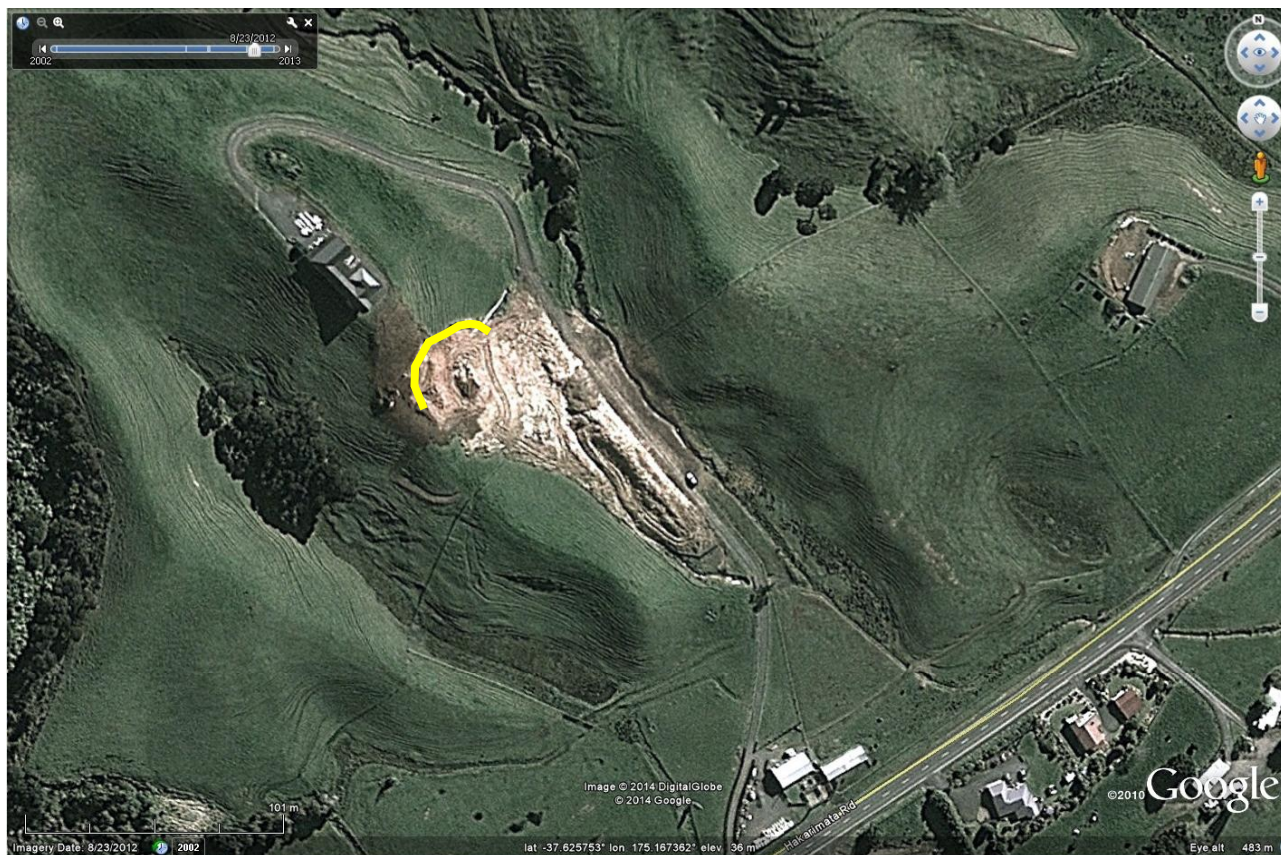
4. This image was taken in August 2012 approximately 6 weeks after the slip occurred. Note the soil has flowed approximately 100 metres from the headscarp. Works have cleared the driveway however surge marks are still visible on the opposite ridge.
