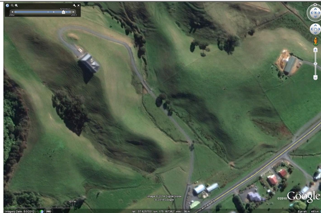
3. By May 2012 a house was relocated to the risge. The image indicates that the driveway did not interfere with the toe of the slope, which subsequently failed in July 2012. The image also indicates that no earthworks were undertaken on the slope.
