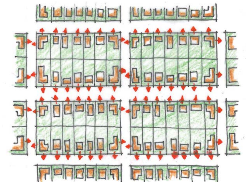
Figure 18. Grid pattern blocks, designed so that all residents have a 'street address' facilitate safer streets and social interaction, while providing potential for good on site amenity.
