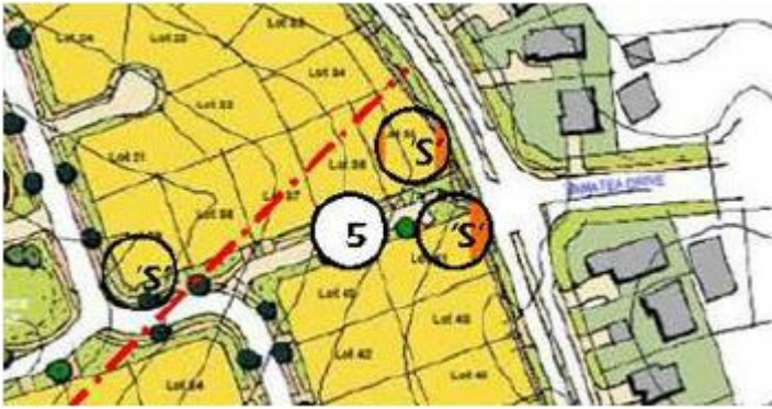
Figure 7: Where an intersection cannot be formed on an arterial road a shared lane with properly formed footpath creates a better pedestrian/cyclist link. Courtesy Kapiti Coast District Council.
