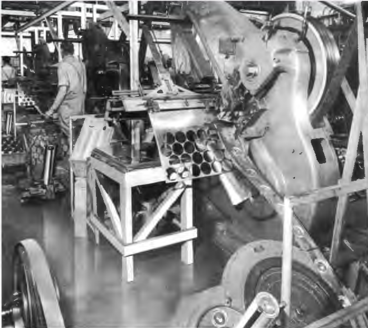
Die cutting presses in operation making the cans.
