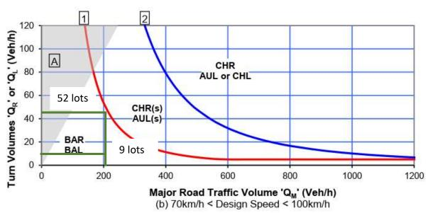
Figure 20: Austroads GTTM Part 6:2020 Figure 3.25 warrant for turn treatments – 70 – 100 km/h
