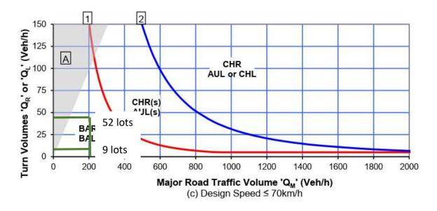
Figure 21: Austroads GTTM Part 6:2020 Figure 3.25 warrant for turn treatments < 70 km/h
