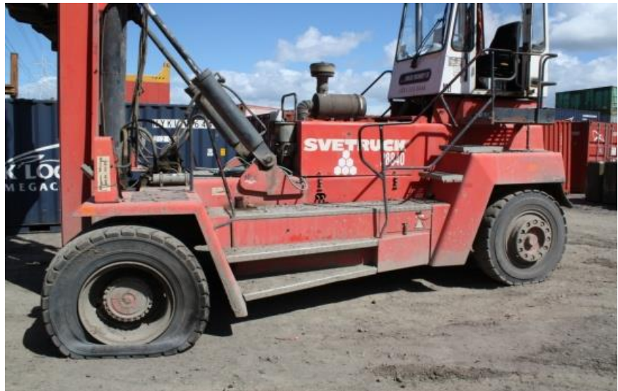
Figure 11: Mobile plant incident flat tyre
