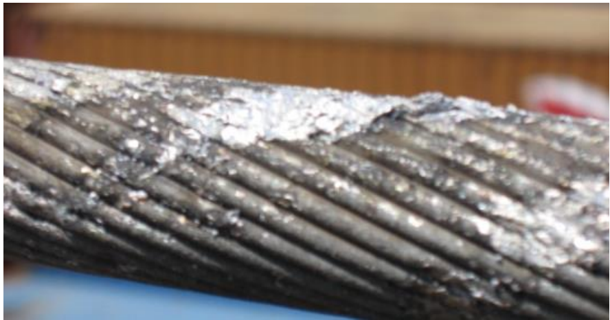
Figure 12: Mobile plant incident – conductor damage
