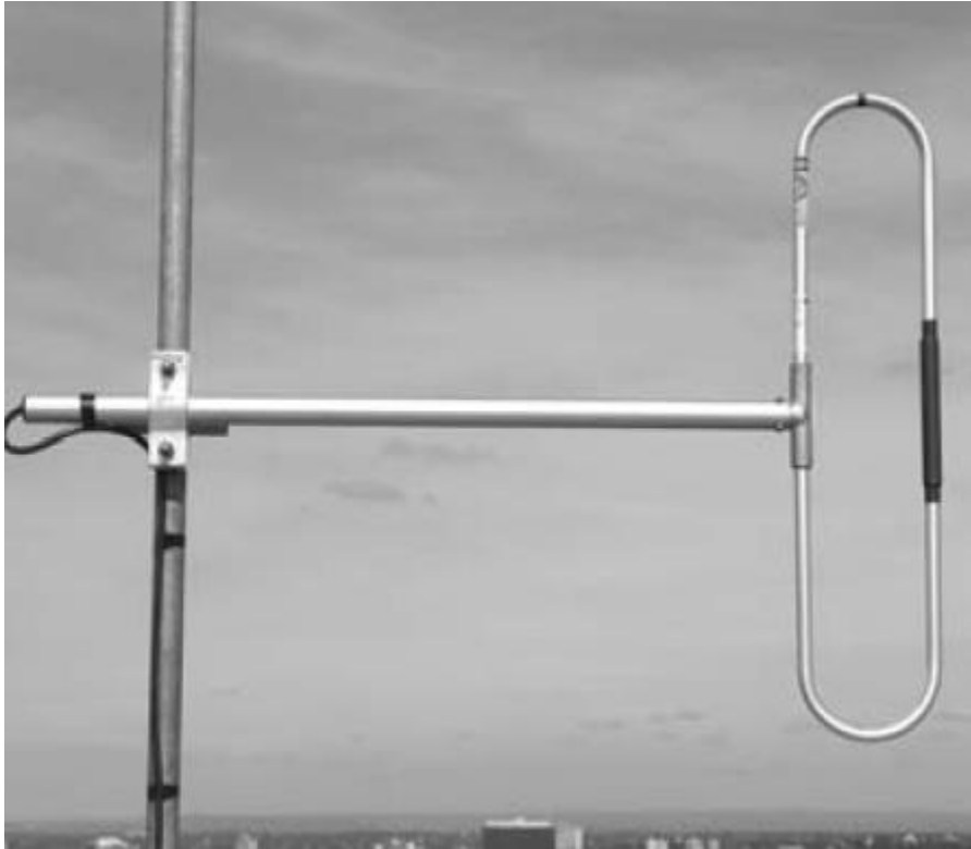
Figure 2: Dipole Antenna example – note minor bulk fo horizontal boom
