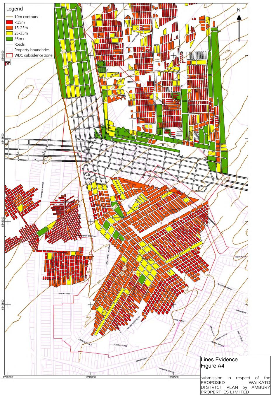
Figure 12. Mine workings with effective width of pillars colour coded, overburden thickness contours.
