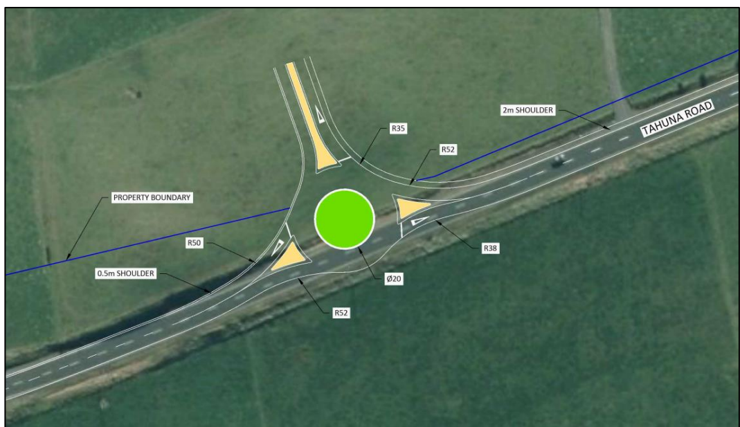
Figure 13: Proposed Intersection Configuration - Access Intersection 2
