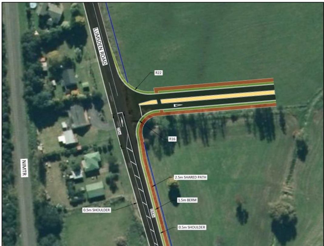
Figure 15: Proposed Intersection Configuration - Access Intersection 4
