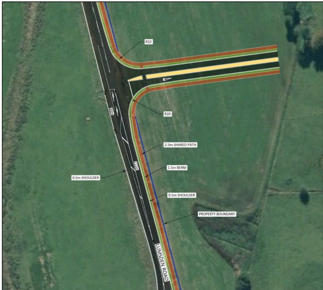
Figure 14: Proposed Intersection Configuration - Access Intersection 3
