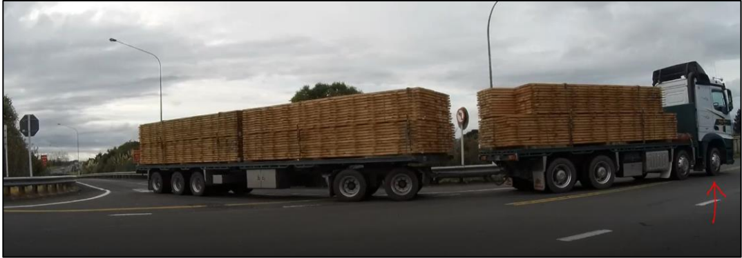
Figure 23: Observed HPMV truck manoeuvre at the southbound off-ramp (June 2020)
