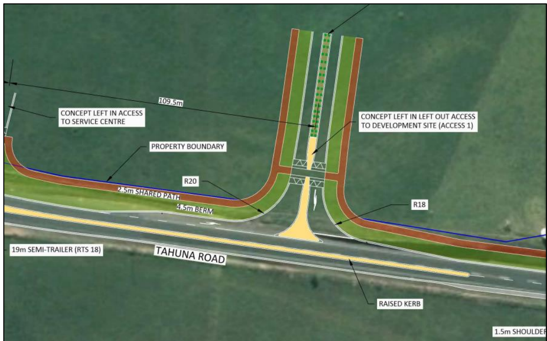
Figure 12: Proposed Intersection Configuration - Access Intersection 1
