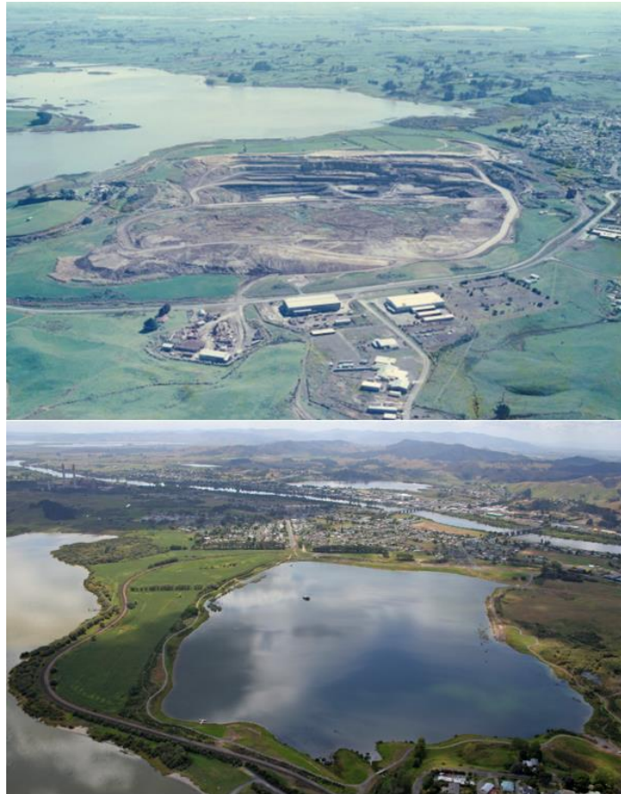
Figure 9 – Lake Puketirini is the mine lake resulting from rehabilitation in the late 1990's of Weavers Opencast at Huntly. It represents the outcome of what was then prevailing best practice rehabilitation and is a valued community amenity (Top - Weavers Opencast 1990; Bottom - Lake Puketirini 2007). The highwall in the top image is steeper than that envisaged for Ohinewai.
