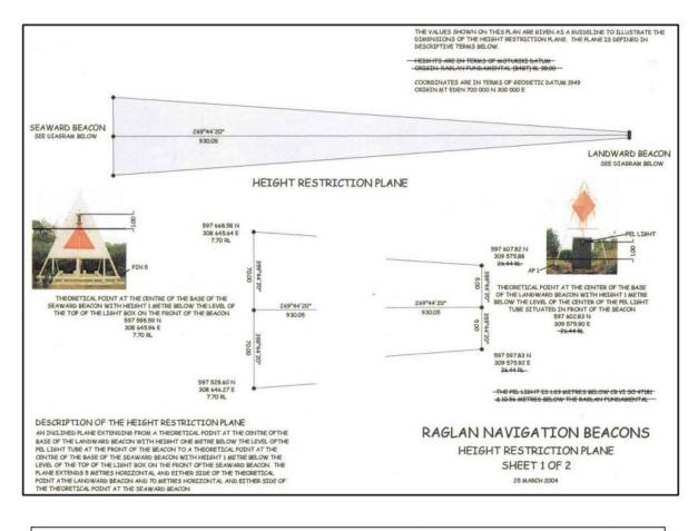
Note: The height of the landward beacon is not fixed in the plan and reference is made to its actual height, whatever that may be at a point in time
