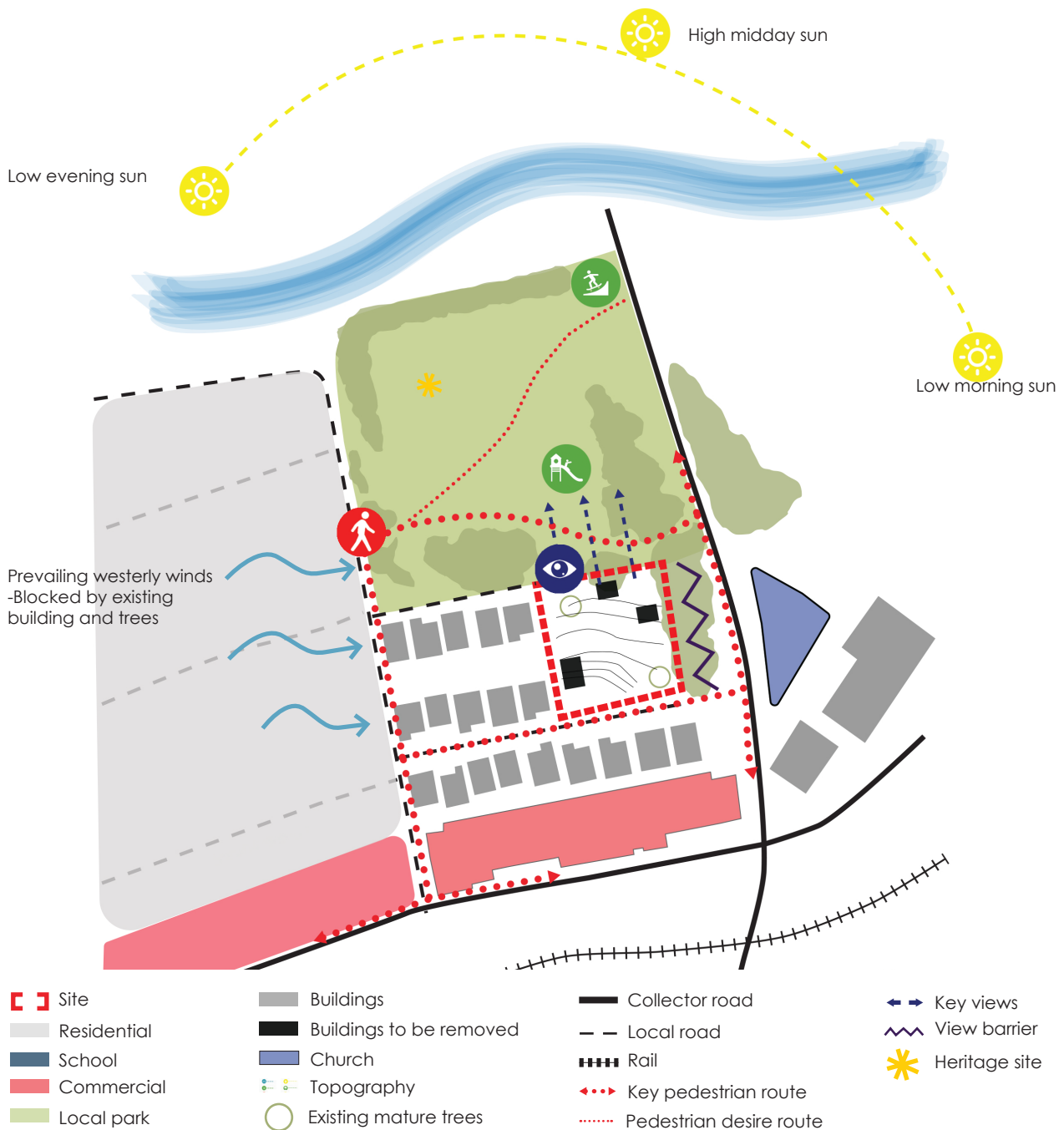
Figure 1. Diagram showing elements that should be considered as part of multi-unit development analysis; the level of analysis will commiserate with the size and location of proposal.
