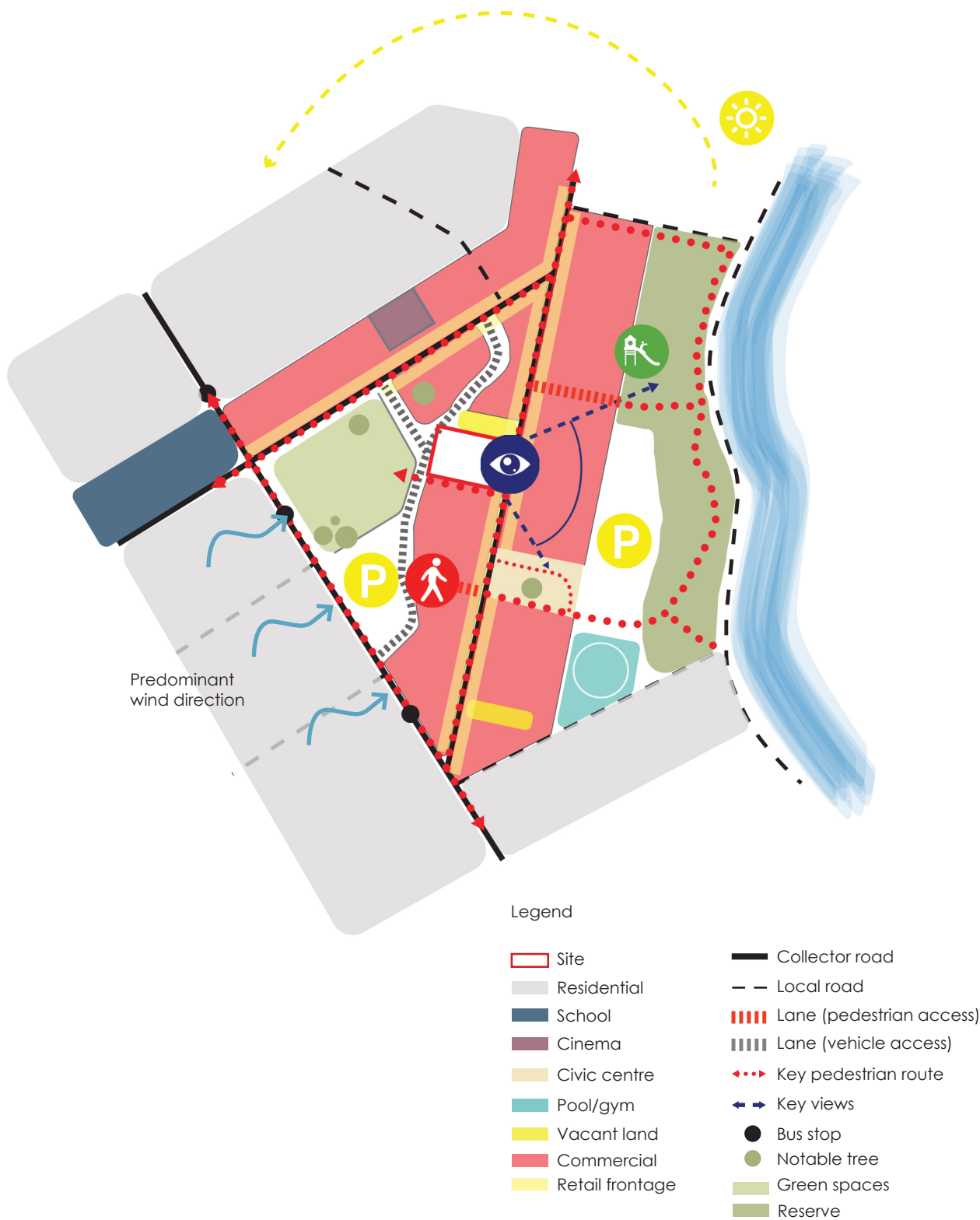
Figure 1. Diagram showing elements that should be considered as part of wider town centre analysis; the level of analysis will commiserate with the size and location of proposed development.
