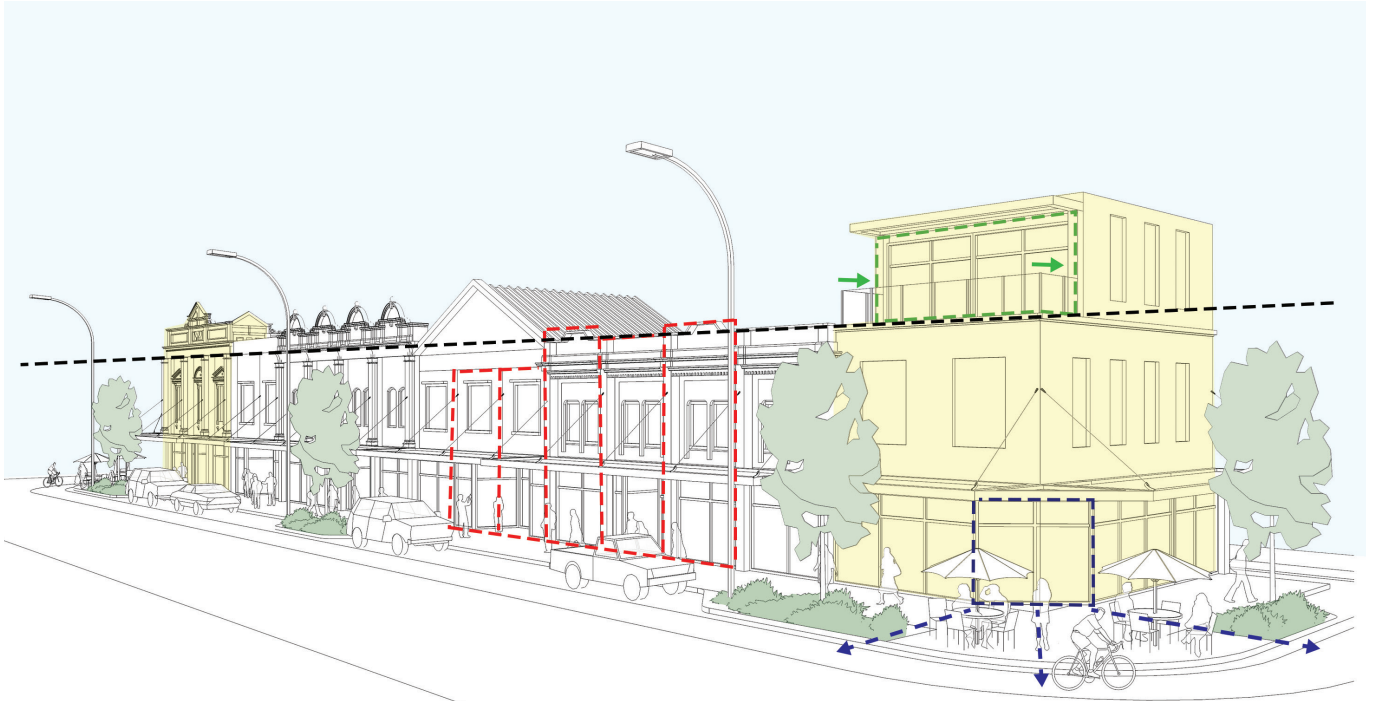
Figure 2. Break up mass of buildings through vertical elements; set back upper stories where appropriate; provide for continuous horizontal elements.
