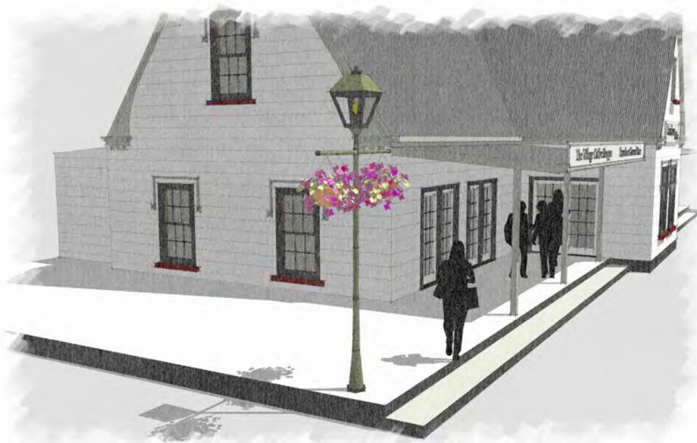
Figure 2. Typical roof design with lean-to verandah configuration
