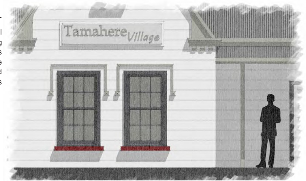
Figure 6. Typical traditional double hung sash windows with decorative mouldings and coloured sills
