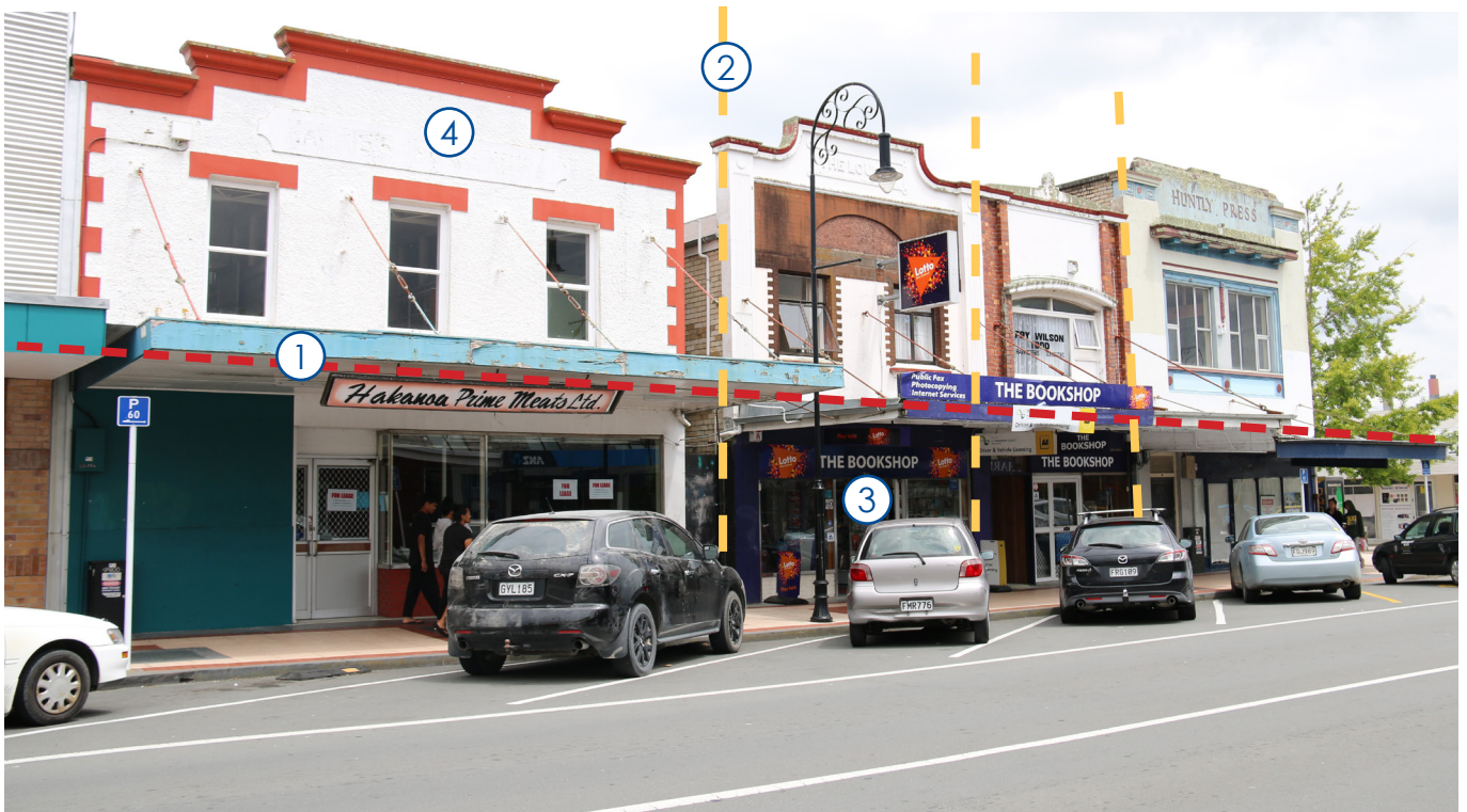
Figure 1. Huntly Town Centre - photograph of Main Street showing key built form outcomes to be incorporated as part of future development within the town centre: (1) consistent verandah line (suspended verandahs); (2) clear vertical differentiation between buildings; (3) large, open, active façades; (4) consistent above verandah parapets with symmetrical detailing and window placement.
