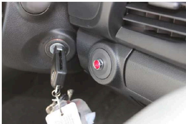
SB-DWL x1: Door open warning light, mounted to the dashboard, with sensors fitted to service body doors.
