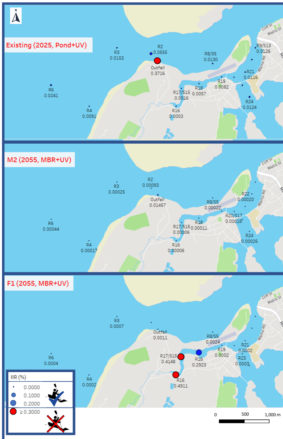
Figure 5. Spatial distribution of child acute febrile respiratory illness risk (based on adenovirus) associated with non-contact recreation at the various exposure sites. Individual illness risk profiles are presented as numbers below the sites. Sample scenarios reflected in plot: Existing (Pond + UV, discharge to existing outfall), M2 (MBR + UV discharge to new outfall), F1 (MBR + UV discharge to Wainui Stream).
