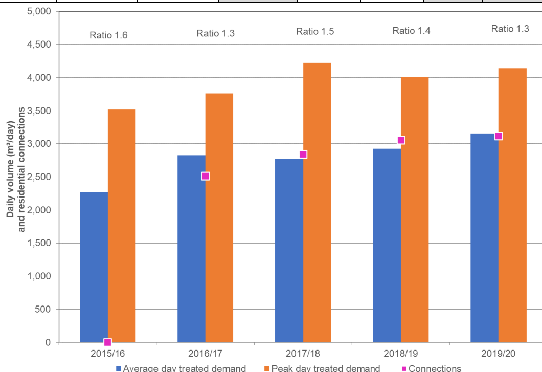
Figure E-30: Ngaruawahia historic annual average daily abstraction and peak day abstraction
