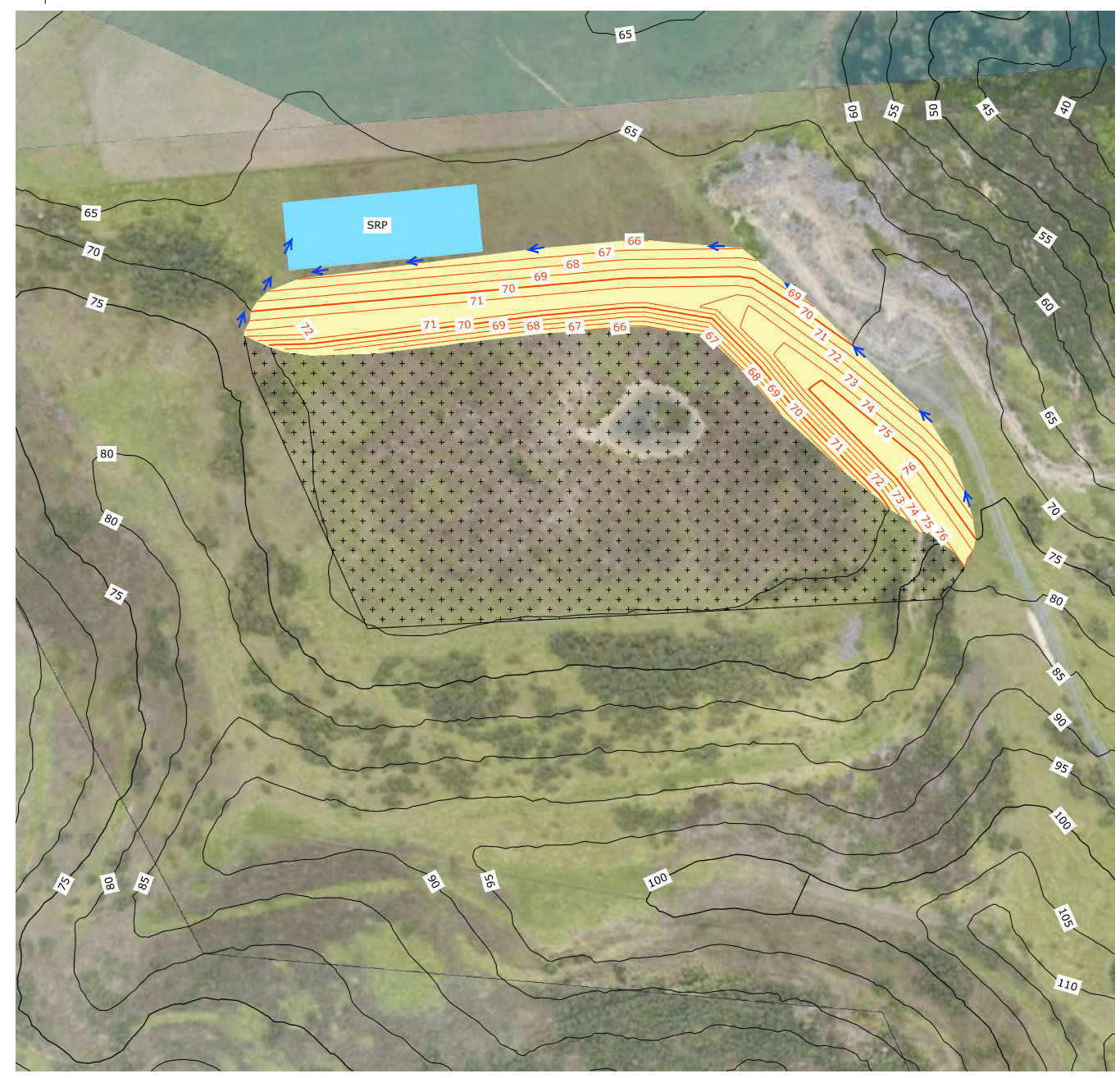
STAGE 1.1 STRUCTURAL FILL (BUND) LAYOUT SCALE 1:2000
