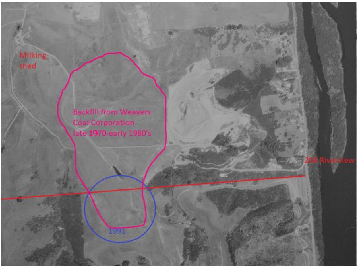
Fig 8. 1991 image illustrating backfill imported from Weaver's pit (Lake Puketirini) with State Coal (Coalcorp).
