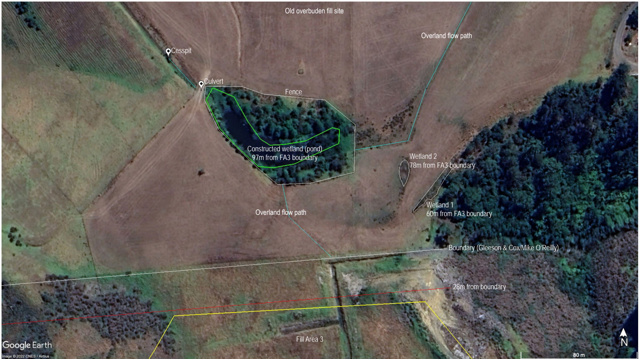
Figure 1: Map of hydrological features and boundaries associated with Fill Area 3, Gleeson Huntly Quarry. Google Earth (February 2019).
