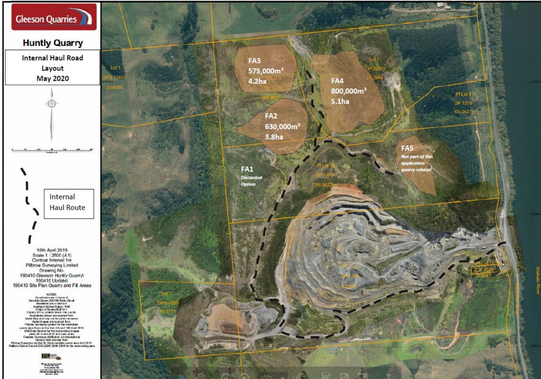
FIGURE 1: INTERNAL ACCESS ROAD AND LOCALITY/CAPACITY OF GULLIES
