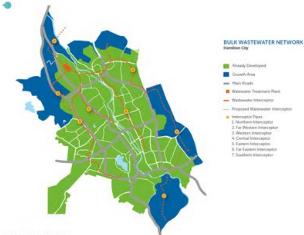
FIGURE SC-6: BULK WASTEWATER NETWORK
