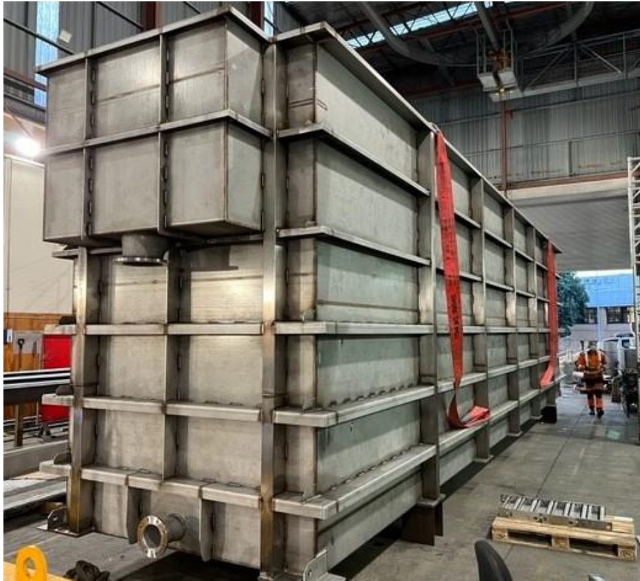
Te Kauwhata WWTP – New MABR Tank
