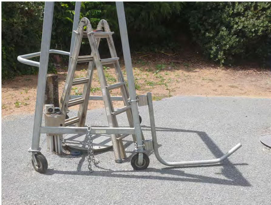
Figure 1. Prototype of outriggers being installed
