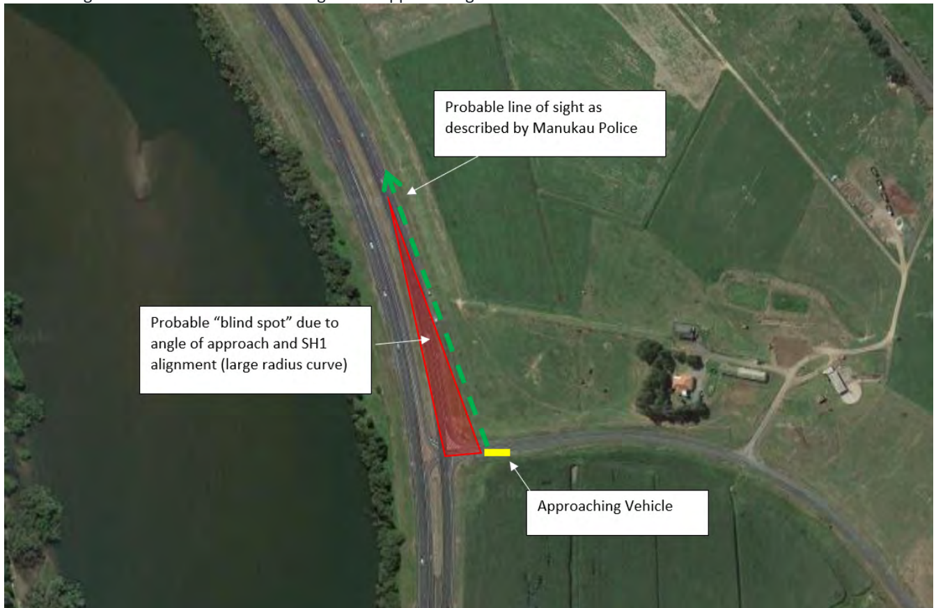
Figure 5: Illustration of probable cause Police of failure to give-way leading to right turn against right side crashes at The Intersection. As described by Manukau Highway Patrol.
