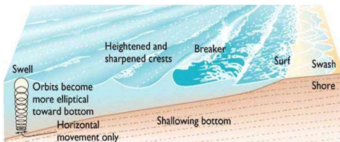
Figure 2.7. Schematic of wave shoaling – as waves enter shallower water their height increase and, the wave length decreases until they become unstable and break
