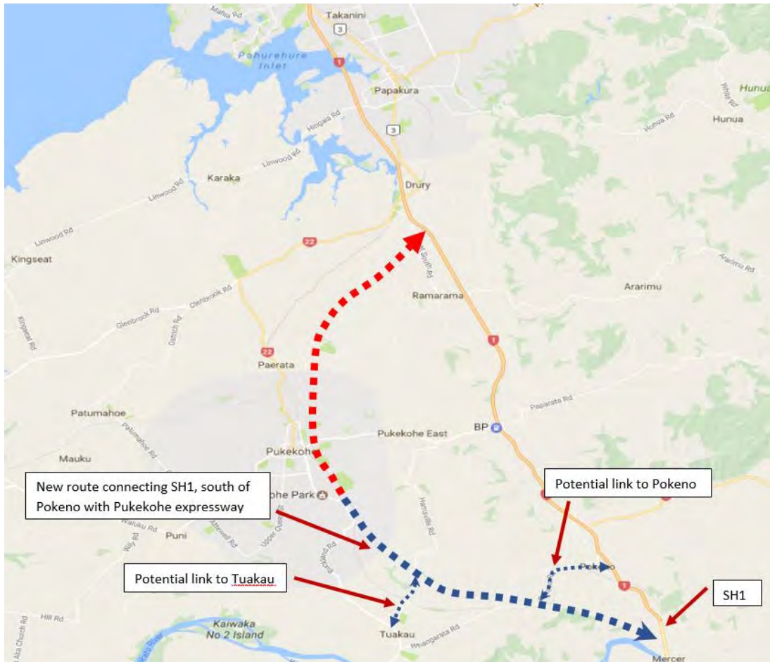
Figure ES1: Possible new Roothing Connection from SH1 south of Pokeno (shown indicatively in blue) to Future Pukekohe Expressway (shown indicatively in red) 1
