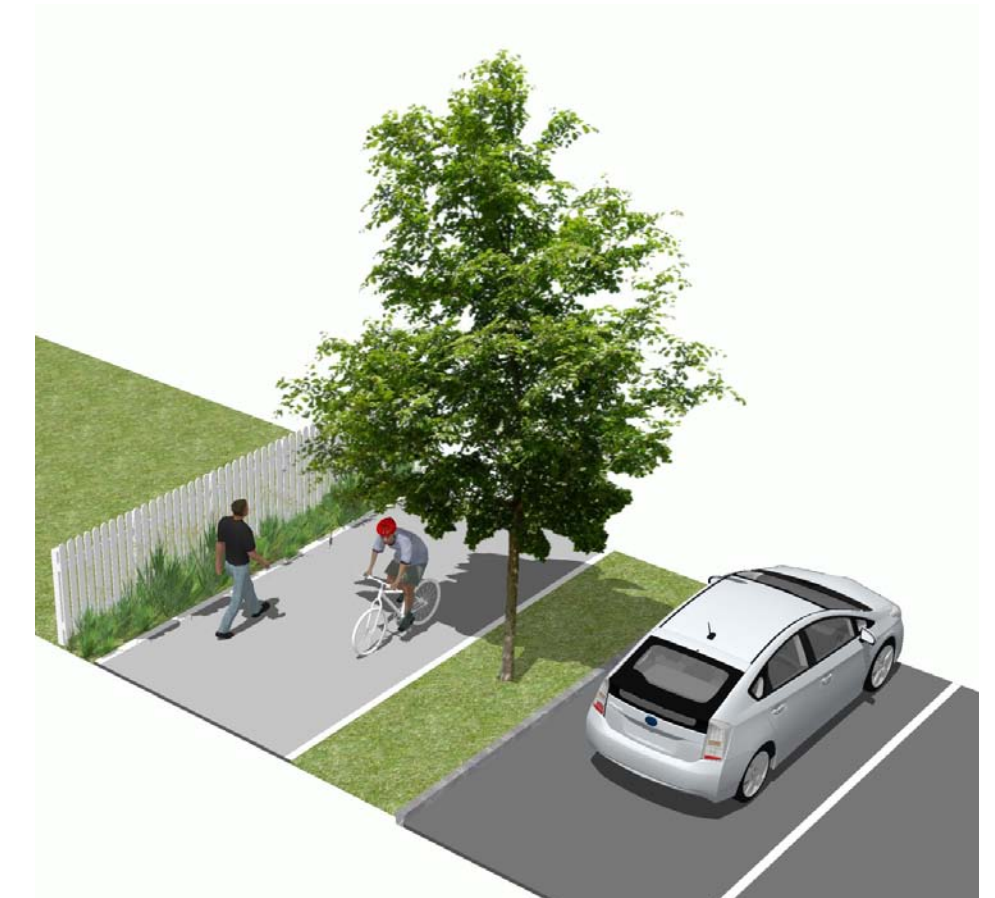
EXPOSED AGGREGATE CONCRETE PATH - 2.5M
