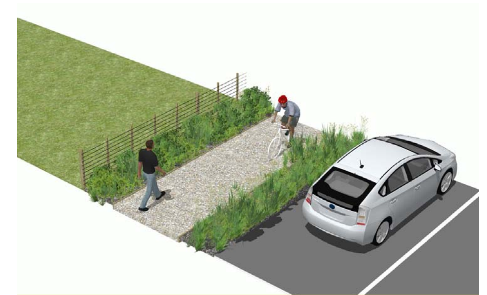
COMPACTED AGGREGATE SHARED PATH - 2.5M
