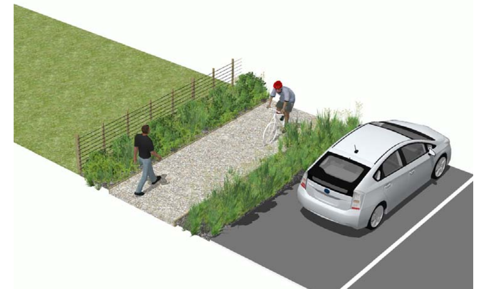
COMPACTED AGGREGATE SHARED PATH (ROAD SIDE) - 2.5M
