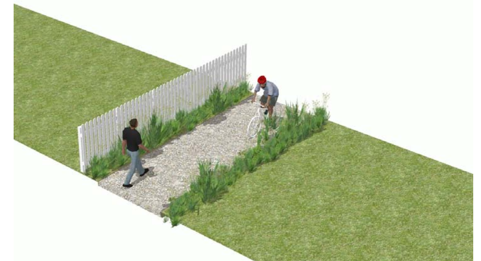
COMPACTED AGGREGATE PATH (OFF ROAD) - 2.5M
