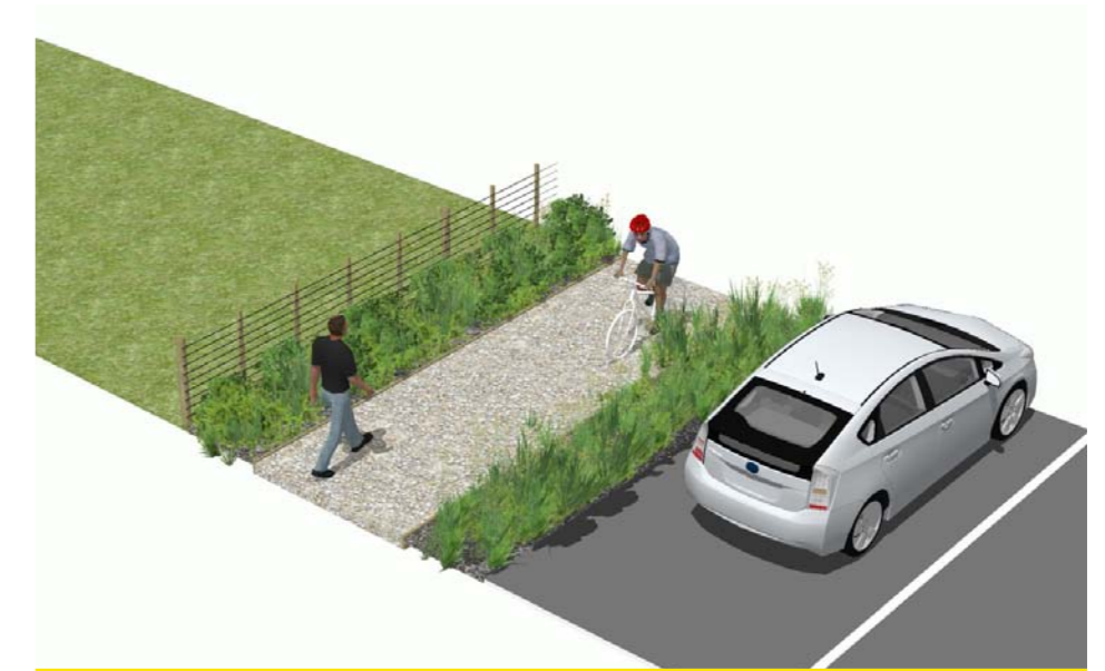
COMPACTED AGGREGATE SHARED PATH - 2.5M
