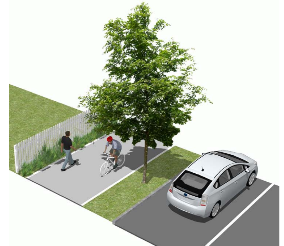
EXPOSED AGGREGATE CONCRETE PATH - 2.5M
