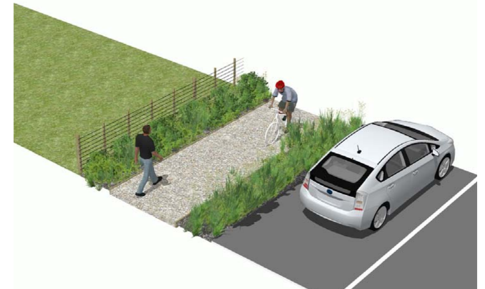
COMPACTED AGGREGATE SHARED PATH (ROAD SIDE) - 2.5M
