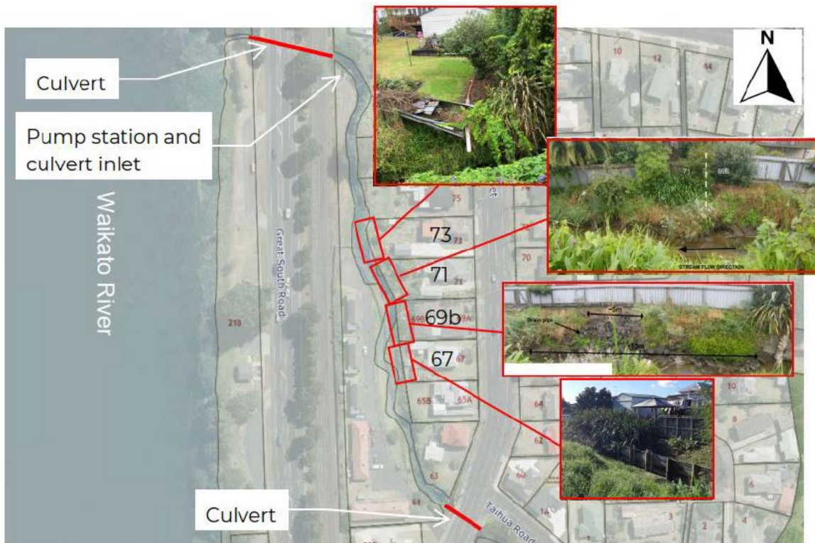
Figure 2 Properties in Hakanoa Street, Huntly experiencing erosion as a result of Hakano Stream (WSP, 2021)
