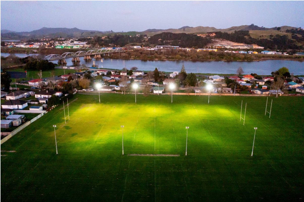
Current lights, showing highly variable light outputs
