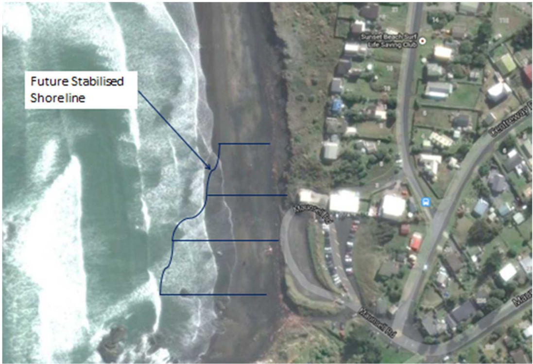
Figure 25 : Diagram of Potential Groins at Port Waikato
