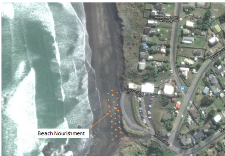
Figure 23: Diagram of Potential Beach nourishment at Port Waikato
