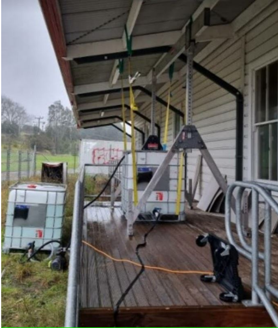
Load testing the portals. Bracing was in place to ensure safety of engineers under the shelter.
