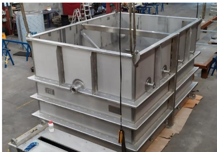
Meremere WWTP – Completed MBR tanks
